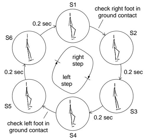
Figure 9. Finite state machine employed for walking.
