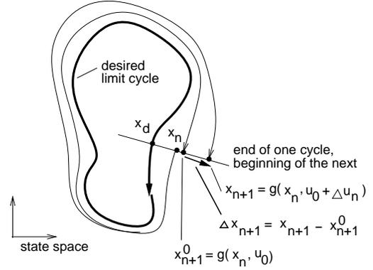
Figure 3. A limit cycle as a discrete dynamical system.
