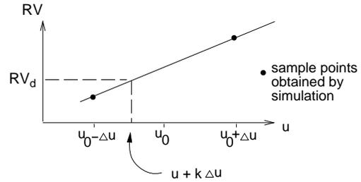
Figure 11. Interpolating for a desired control perturbation.
