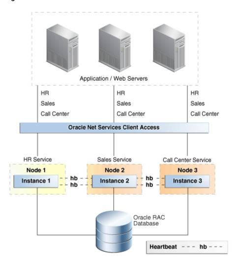
Figure 3-2 Oracle Database with Oracle RAC Architecture
