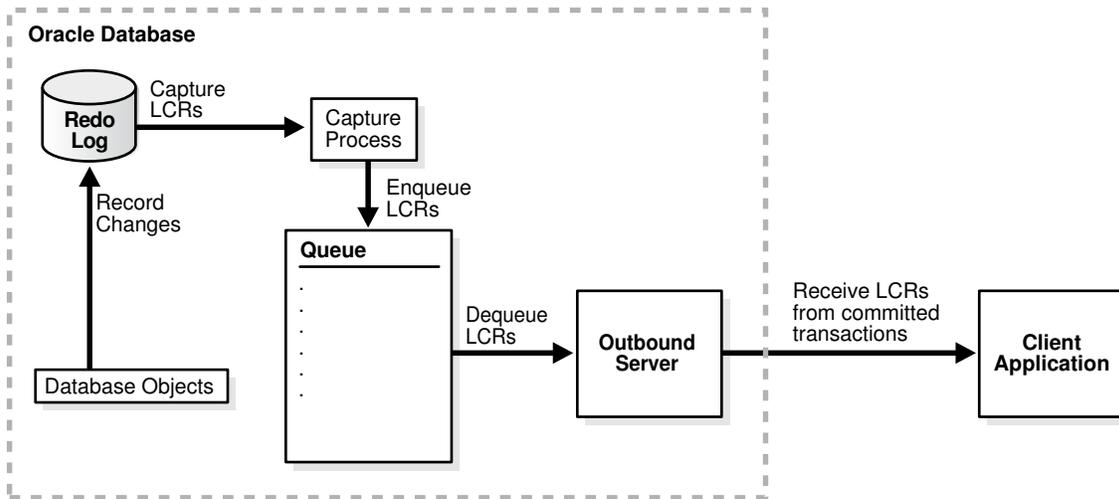
Figure 4-2 Local Capture and Outbound Server in Different Databases
