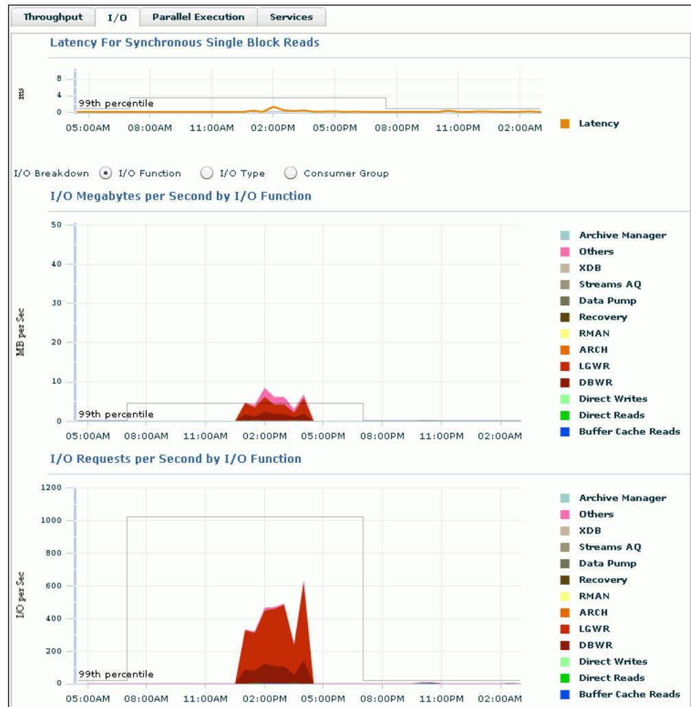
The Latency for Synchronous Single Block Reads chart shows the total perceived I/O **latency** for a block read, which is the time difference between when an I/O request is submitted and when the first byte of the transfer arrives. Most systems are performing satisfactorily if latency is fewer than 10 milliseconds. This type of I/O request is the best indicator of I/O performance for the following reasons:
