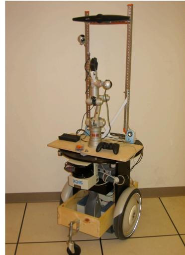
Figure 1: The STAIR robot.
