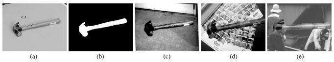
Fig. 3. Our synthetic data system: (a) Object view as seen by the capturing camera, with fiducial marking. (b) Mask extracted from the green-screen image. (c),(d),(e) Synthesized positive examples.
