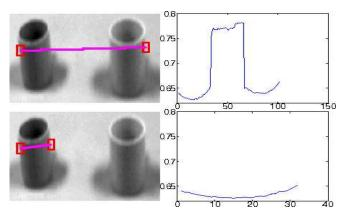
Fig. 7. Depth variation features: we can use the changes in the depth as a feature. Top row: a bad pair and corresponding change in depth taken from the connecting line (magenta). Bottom row: a better pair and the corresponding change in depth. Notice that the depths change more in the bad pair than in the good pair.
