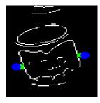
Fig. 3. Edge map (white), contact points (green crosses), and finger placements (blue circles). This edge map is extracted from the mug picture in Figure 1. See text for more details.
