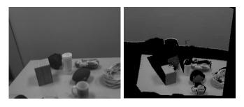
Fig. 2. Image data and depth data captured by our robot. Left: visible light image data. Right: depth data (note: missing back face of objects).
