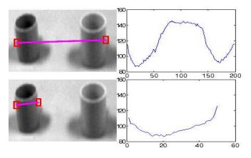
Fig. 8. Pixel intensity variation features: we can use the changes in the pixel intensity as a feature. Top row: a bad pair and corresponding change in pixel intensity taken from the connecting line (magenta). Bottom row: a better pair and corresponding change in pixel intensity. Notice that the pixel intensities change more in the bad pair than in the good pair. Note that there are more points in the x-axis of this figure than the previous figure because of missing depth readings.
