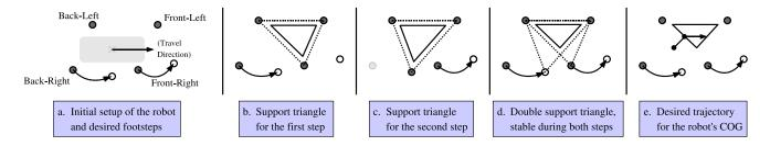
Fig. 4. Planning of the COG trajectory for a sequence of two steps.
